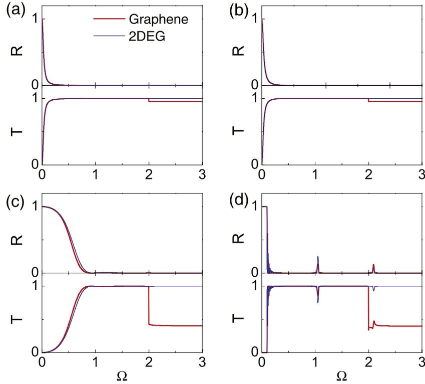
**Figure 5.** Comparison of reflection and transmission spectra between graphene and 2DEG layers at normal incidence. (a), (b) Two graphene and 2DEG layers with  $d = 0.1\hbar c/\mu$  and  $d = 3\hbar c/\mu$ , respectively. (c), (d) 40 graphene and 2DEG layers with  $d = 0.1\hbar c/\mu$  and  $d = 3\hbar c/\mu$ , respectively.
