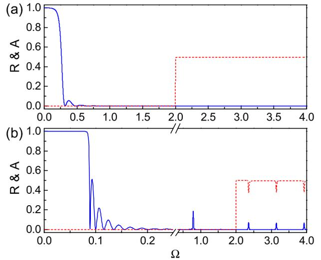
**Figure 4.** The reflectance (solid line) and absorbance (dashed line) spectra of 30 graphene layers at normal incidence. (a)  $d = 0.4\hbar c/\mu$  and (b)  $d = 4\hbar c/\mu$  (corresponding to  $0.132$  and  $5.26 \mu\text{m}$  for  $\mu = 0.15 \text{ eV}$ , respectively).
