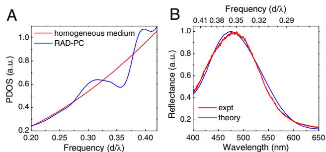
**Fig. 2.** (A) Calculated PDOS for the model RAD-PC as a function of reduced frequency  $d/\lambda$ , where  $d$  is the rod length and  $\lambda$  is the vacuum wavelength. The PDOS for a homogeneous medium with refractive index  $n = 1.23$ , a volume-weighted average, is also given for comparison. (B) Normalized calculated and measured reflection spectra under normal incidence. The calculations were based on observed  $d = 170$  nm.
